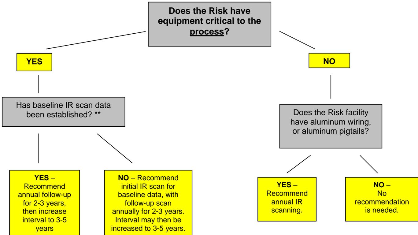
\*\* Baseline data is the original data received from an IR scan of the critical process equipment reflecting optimal operation of the equipment. If the initial scan has revealed abnormalities requiring mitigation, a timely follow-up scan must be conducted once the repairs are completed. Data from future scans is then analyzed in comparison to the baseline data to reveal potentially hazardous changes.
