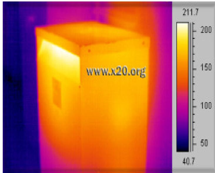
NFPA 70B indicates that routine IR scanning should be conducted annually for all critical process equipment. The applicable sections are as follows:
